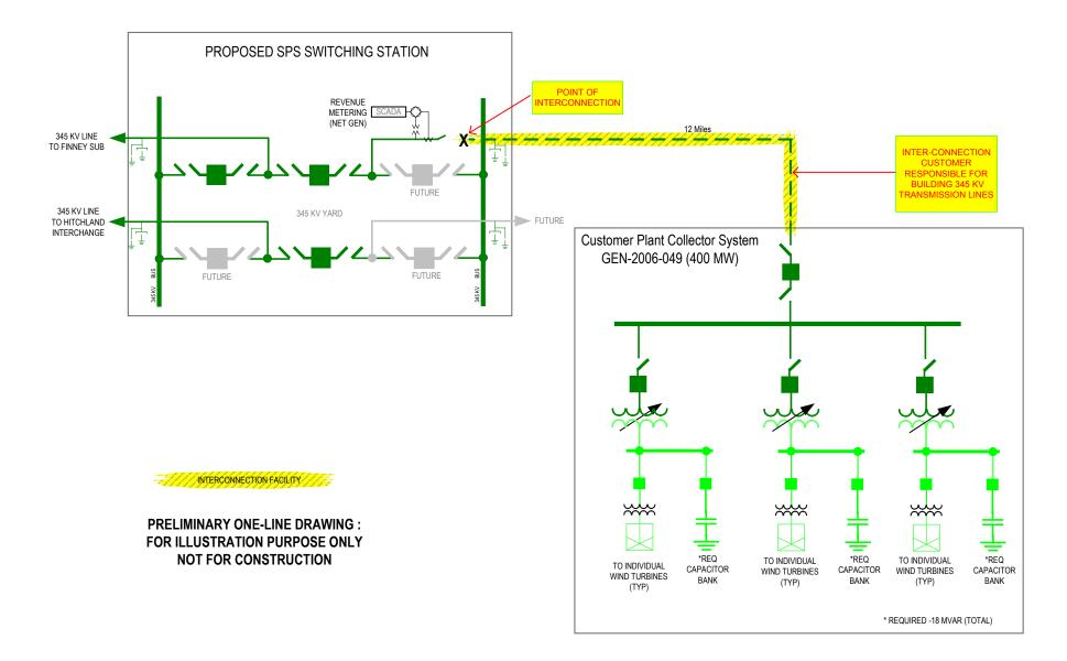
Figure A- 2 One-line Diagram of Proposed SPS Switching Station to Customer Interconnection Facility
